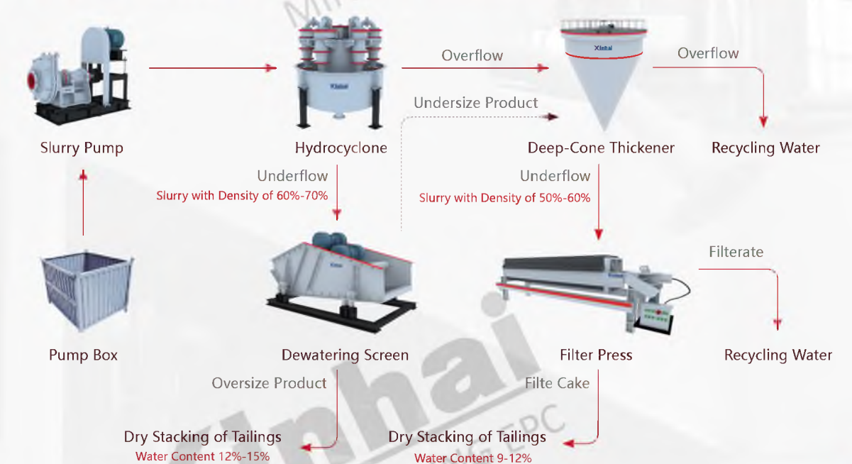
© Tailings Dry Stacking Flowsheet
